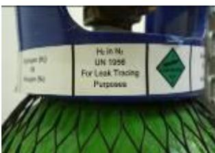
A trace of hydrogen (5% max. for safety reasons) or helium (10-30%) with the nitrogen will enable leaks to be found at a lower pressure. A suitable electronic detector must be used – your standard detector is not sensitive to hydrogen or helium. Nitrogen can be supplied with a trace of hydrogen (as shown in the photo) or helium specifically for leak testing.
